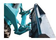
Adapt to international common quick coupler, fast change various kinds attachment. Majority of attachments can be used in Sunward skid steer loader.
